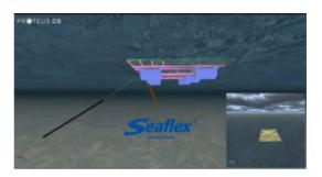
The modelling of the interaction between the floating farm and the swell has been part of the tasks of the WP2 of the project. It allowed to understand the behaviour of the structure under extreme environmental conditions and the influence of the type of mooring on it.
