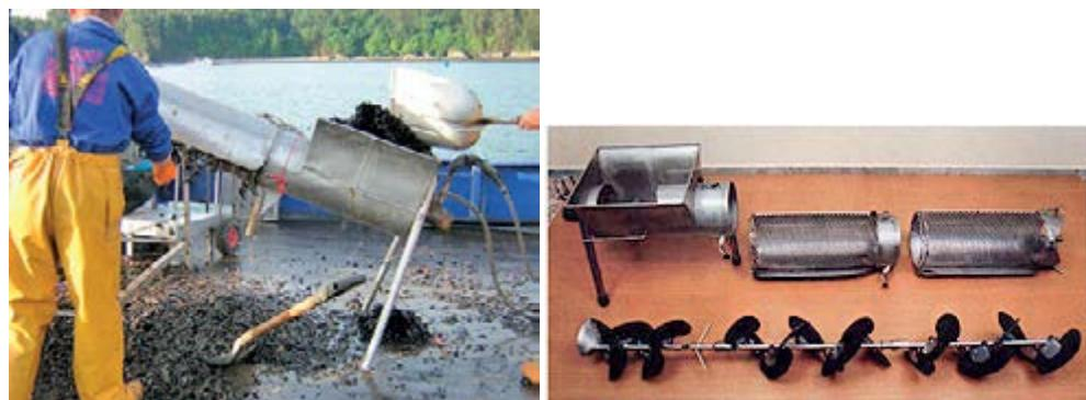
*Figure 15. Separation of the mussel from the rope and parts of a sheller*
