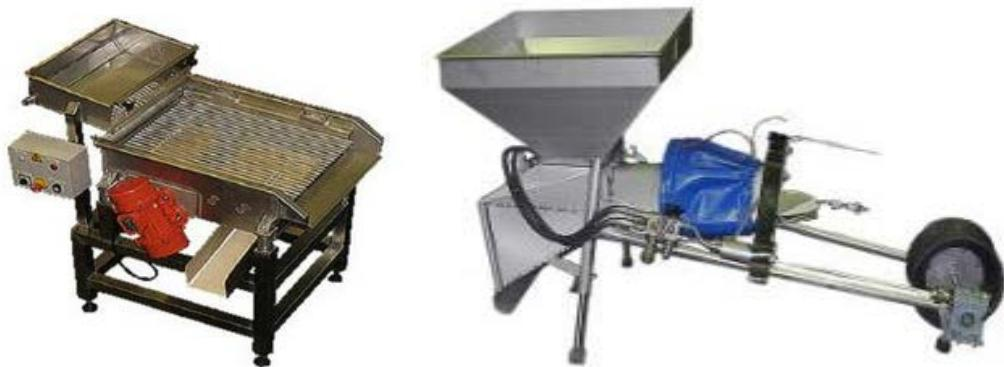
Figure 22. Left: Selector table with vibrator from the company Taller Dios (Illa de Arousa). Right: Unfolding machine with two hydraulic engines. Taller Dios (Illa de Arousa).
