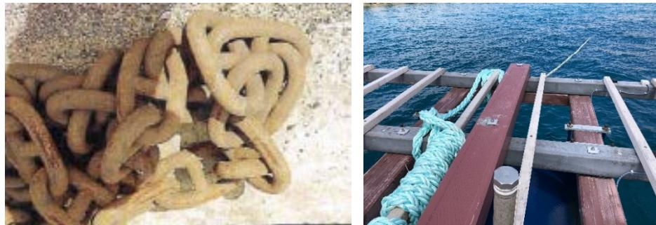
*Figure 60. Shackle chain and example of the necklace of a nylon rope in a Formex®Mixta raft*
