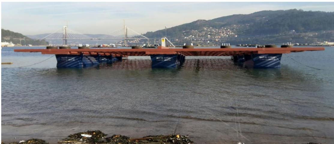
*Figure 14. Same raft as in figure 13, but two days later, with higher tide. The two mooring ropes to avoid a possible drift of the module can be seen*
