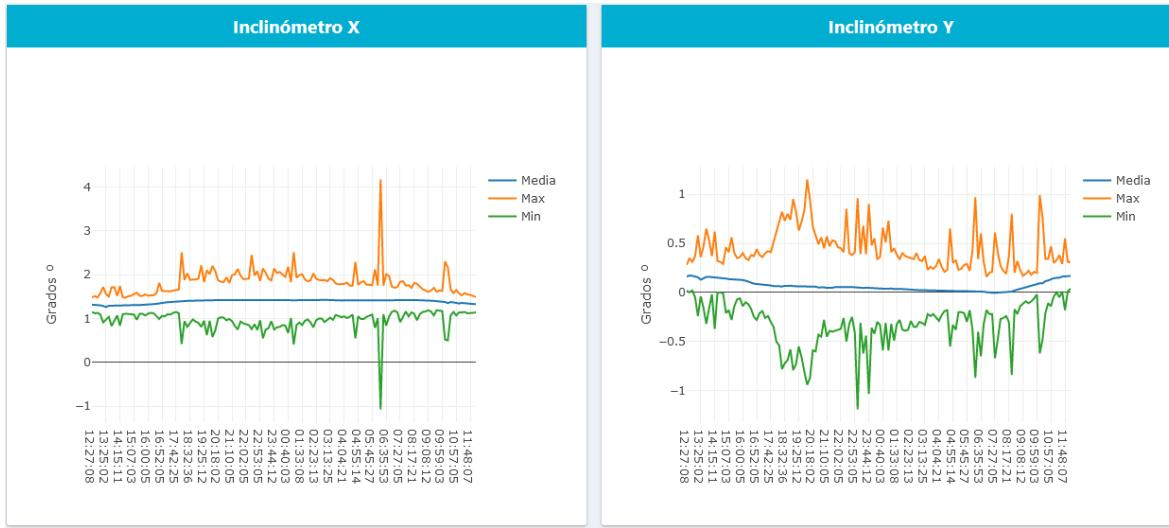
*Figure 20. Detail of the display of the inclination in X and Y axis of the module. Last 24 h*
